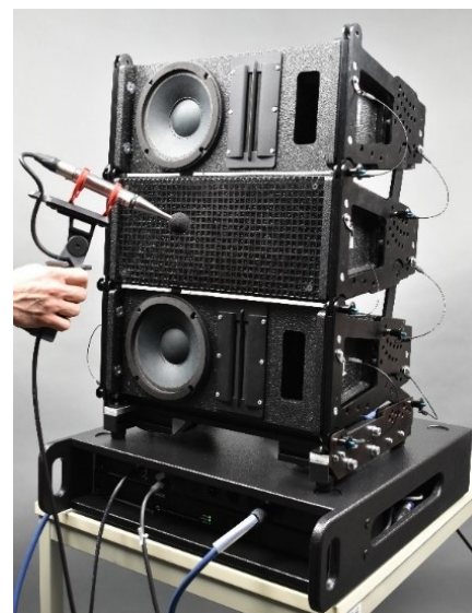
Figure 3: Fast and cost-efficient quality check of rental Sound Reinforcement Equipment using streaming V/I amplifiers and QC Stand-alone Software.
