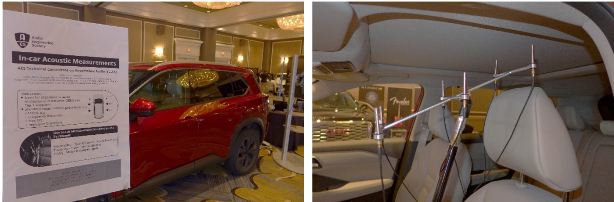
Figure 4+5: Acoustic in car test setup using microphone array on AES Automotive Audio conference in Detroit July 2022.
