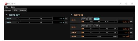
**Note**: the ASIO input/output channels are assigned in the order of appearance in the control panel.
