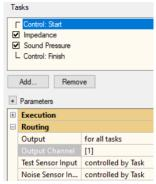
• Now set the input channels in the Impedance and Sound Pressure task (remember that the ASIO channel number corresponds to the order of hardware input channels as shown in the AIO Control Panel)
