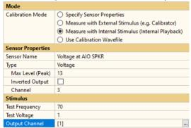
• Enter the value displayed in the AIO Control Panel (VMON) or use an external multimeter for more accurate readings
