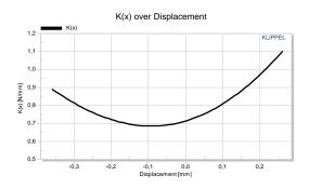
Figure 4: Nonlinear Stiffness K(x) of the micro-speaker diaphragm
