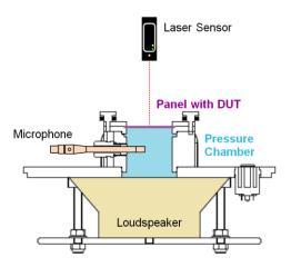
Figure 5: sectional drawing of micro suspension part measurement (MSPM)
