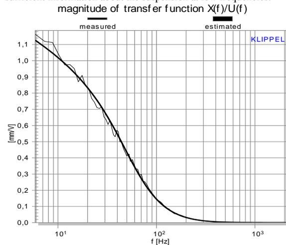
Fig. 5: Transfer function  $H_x$  (measured / estimated with creep model)
