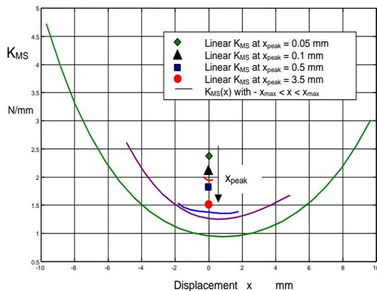
Fig. 13: Linear stiffness  $K_{MS}$  and nonlinear stiffness  $K_{MS}(x)$  of mechanical suspension measured at different amplitude levels
