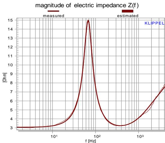
Fig. 3: Measured and estimated impedance
