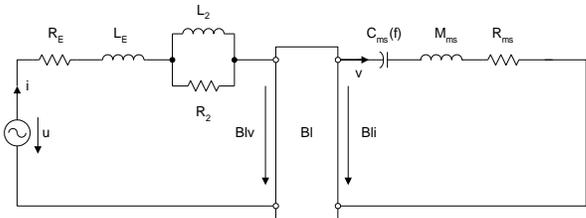
Fig. 1: Linear loudspeaker model
