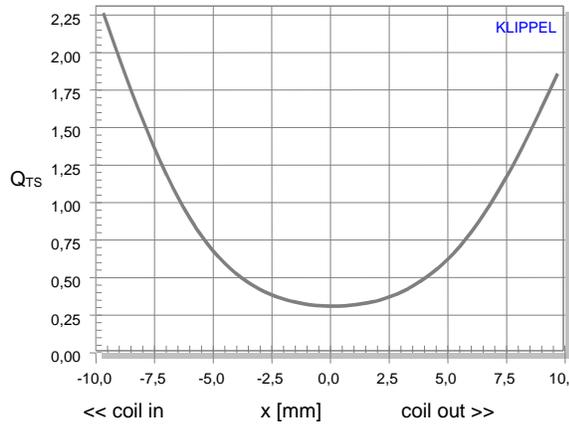
Fig. 12: Total loss factor  $Q_{TS}(x)$  versus displacement  $x$
