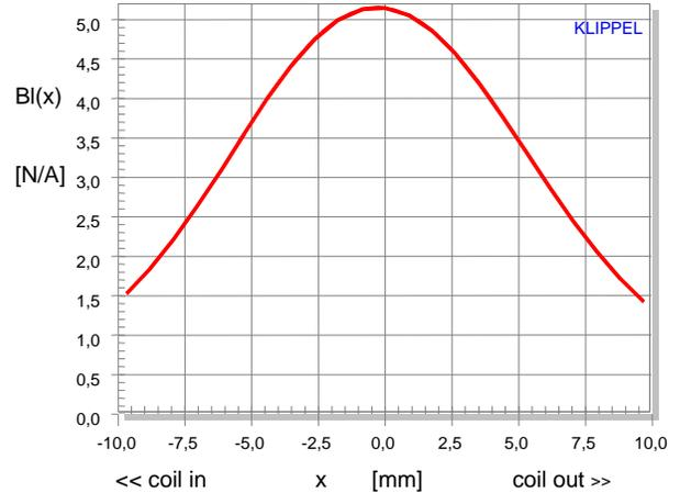
Fig. 10:  $Bl$ -product versus voice coil displacement  $x$
