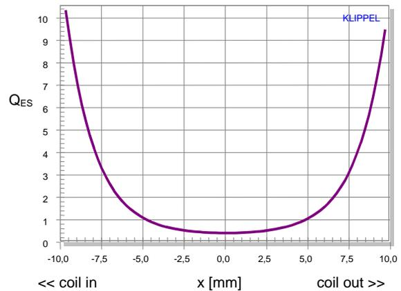
Fig. 11: Electrical loss factor  $Q_{ES}(x)$  versus displacement
