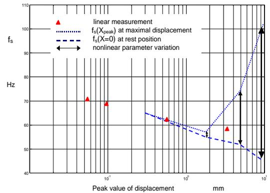
Fig. 14: Resonance frequency  $f_s$  of the driver versus peak value of displacement
