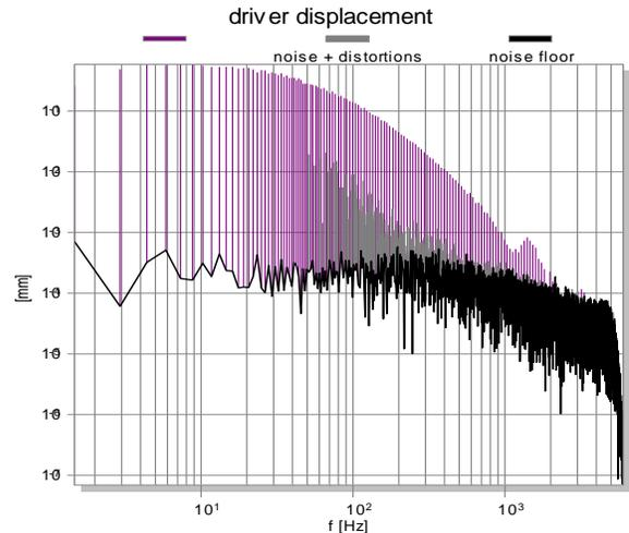
Fig. 9: Spectrum of the laser sensor signal
