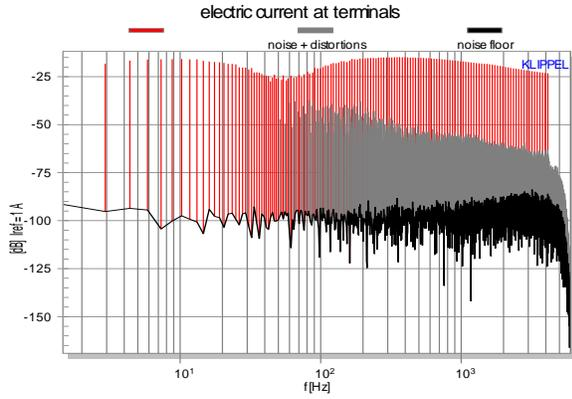
Fig. 7: Spectrum of the current sensor signal
