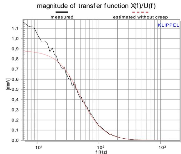
Fig. 4: Transfer function  $H_x$  (measured/estimated without creep model)
