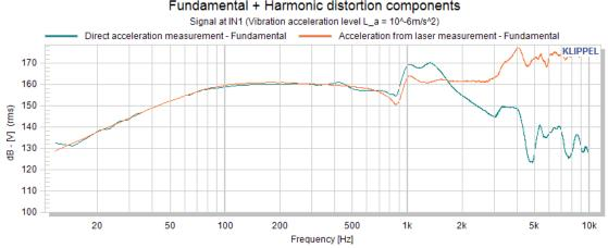
You can see that both curves are matching quite well up to about 600 Hz. Above this frequency the directly measured acceleration starts to rise above the calculated acceleration before it decreases with about 12 dB per octave while the calculated acceleration stays stable until the cone breaks up above 3 kHz.
