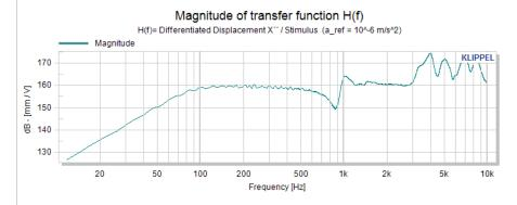
The *PPP* template may also be used for calculating the acceleration in  $[m/s^2]$ , but as already mentioned the absolute acceleration from the fundamental curve is not usable. Thus, the *PPP* template has to be modified for using the magnitude of the transfer function instead. Please refer to the *PPP* manual on how to change the curve input C1.
