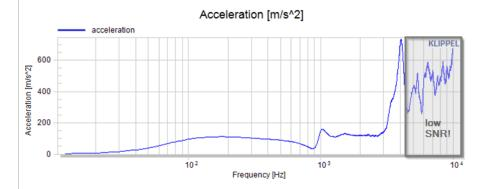
The peaks in the calculated acceleration above 3 kHz are due to the break up modes of the loudspeaker cone. This is a normal behavior of the loudspeaker which can be investigated in more detail using the KLIPPEL Scanning Vibrometer (SCN).
