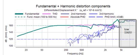
**NOTE:** Since the physical context of differentiating the fundamental twice could not be covered by the reference curve, the shown y-axis label dB - [mm] (rms) is not correct. It should be  $dB - [m/s^2]$  (rms) instead.
