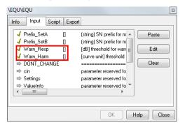
The unit of the entered values is the unit of the measure (response or harmonics). Response is always in dB, harmonics are either in dB or in percent.
