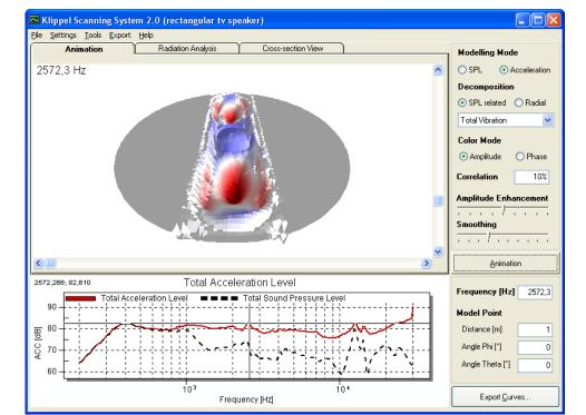
The vibration behavior can be studied over the complete measured frequency range. Peaks in the accumulated acceleration level curve indicate distinct vibration modes.
