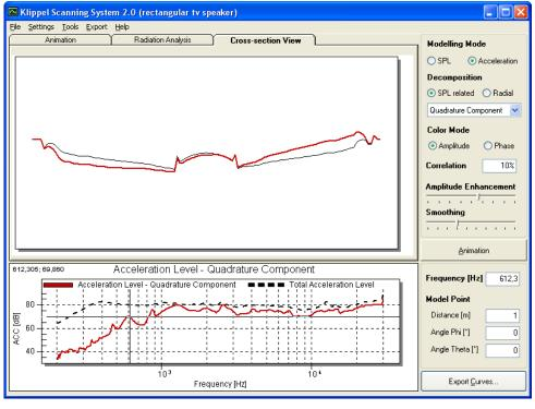
Peaks in the quadrature component curve of the acceleration level indicate vibration modes which do not contribute to the sound pressure output at the selected observing point in the far field, especially rocking motion at lower frequencies.
