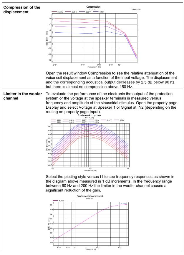
Selecting the plotting style versus voltage U1 and logarithmic Y-axis on property page Display to see the input-output characteristic of the limiter at the critcial frequency of 76 Hz as shown in the diagram above. For small input voltages (< 200 mV) there is a linear relationship between input and output but the maximal output is limited to 400 mV.
