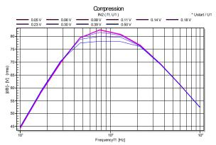
Open the result window Compression to see relative attenuation (-5 dB) of the transfer response at 80 Hz.
