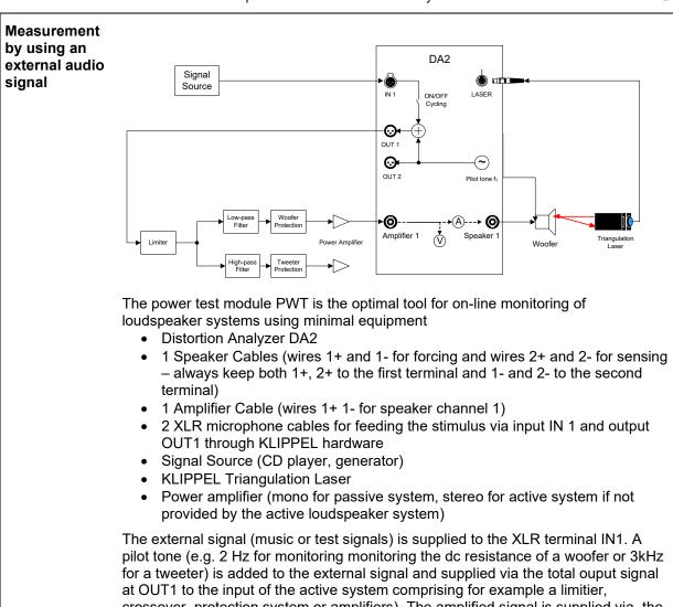
crossover, protection system or amplifiers). The amplified signal is supplied via the voltage and current sensors in the DA2 to the speaker terminals using the Speakon connectors Amplifier1 and Speaker 1.
