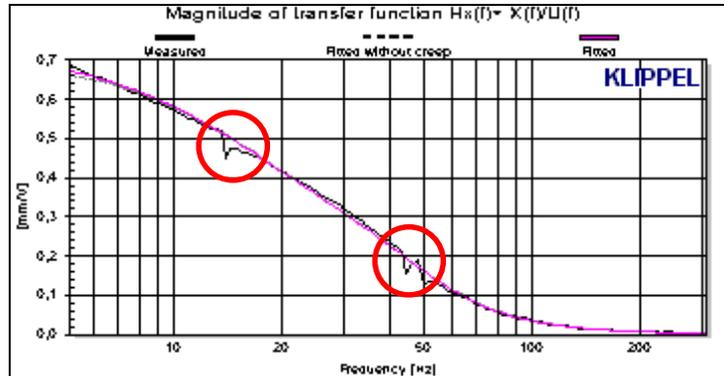
Try to damp the resonances if they are significant. Make sure that your clamping mechanism is appropriate for the driver size. See our product list for clamping and driver stand offered by us.
