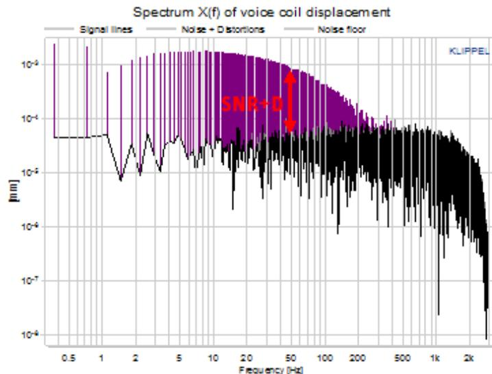
SNR+D of the displacement should be at least 20 dB. If it is too low try to increase averaging and/or the excitation level. Check the impact of the changes to the current spectrum. Readjust the excitation level if necessary.
