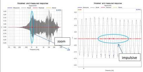
In contrast to the above results there are also some cases where noise corrupts the measurement which sometimes has parasitic influence on the rub & buzz measure. In this case only reviewing the *Residual* curve may show a root cause. In the below picture you clearly see that there is no impulsive distortion but only fluctuating noise.
