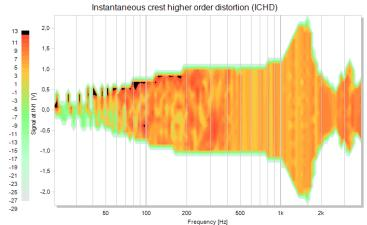
Please note that there is a 180° phase shift between displacement and microphone signal (for a loudspeaker that is measured in free air). You can also check this when comparing the waveforms of displacement and microphone signal in the windows Y1 (t) and Y2 (t) (in the picture below). Thus you will get the black spots of high ICHD values at the positive maximum in this example (according to the negative peak displacement).
