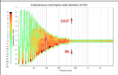
The result window *Instantaneous Distortion 3D* shows the crest factor ICHD (as color) versus voice coil displacement (y axis) and frequency (x axis). This reveals valuable information about the location of the R&B defect. Black spots at frequencies 20-200 Hz and for negative voice coil displacement indicate a voice coil rubbing maybe caused by a tilting of the voice coil.
