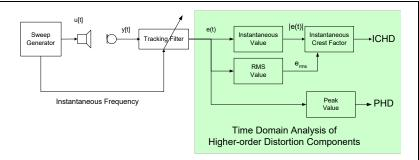
The rub & buzz detection algorithm is based on a time domain analysis to overcome the disadvantages of the THD measure and to show impulsive distortion at high temporal resolution.
