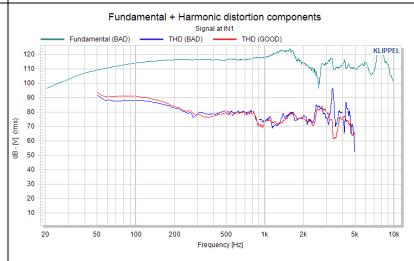
For comparison the THD curves of a good and a bad driver are presented. It is obvious that the THD is not a suited measure to describe and detect rub & buzz phenomena. The regular distortion, caused by motor and suspension nonlinearities, mask the much smaller rub & buzz distortion.
