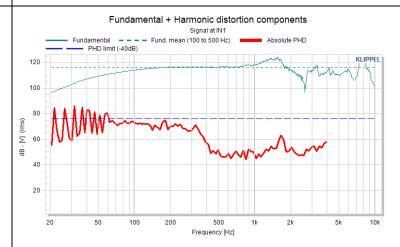
The window *Fundamental* + *Harmonics* shows the Peak value PHD of the harmonic distortion. The PHD is higher than the allowed limit value for frequencies at 20-150 Hz where the crest factor is above the limit. The impulsive distortion has a high impact on sound quality.
