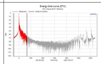
Using the two markers some region of the ETC can be selected for Analysis. In this application the marker positions are not critical, as long as the main impulse is inside the window (important for time delay calculation). However, for separating linear and nonlinear response it is good practice to set the left marker at the left border and the right marker in the minimum of the ETC (use Shift and CTRL + Mouse click).
