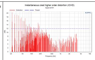
The ICHD is the instantaneous crest factor of the residual e(t). It quantifies the peaky-ness of e(t) and reveals the fine structure of the rub & buzz distortion.
