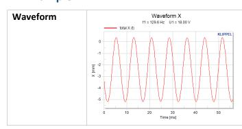
After pausing the measurement, the result window *Waveform Y2* shows the displacement versus time of the last measured point. The DC offset which exceeds the fundamental component shifts the coil out of the gap.
