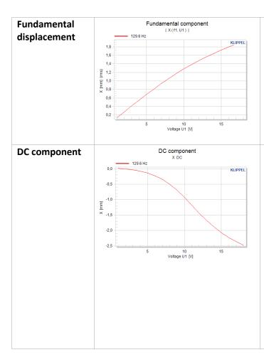
The result window *Fundamental* shows the rms displacement versus amplitude  $U_1$ . At higher amplitudes ( $U_1 > 4 \ V \ rms$ ) there is a distinct compression of the output amplitude because the coil is moved out of the gap. The fact that the fundamental component is plotted in mm (rms) while the DC component is plotted in mm (peak) is no problem for the calculation of  $I_{DC}$ .
