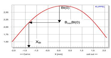
For the particular driver in the example the peak displacement  $X_B$ = 1.38 mm due to force factor using a limit  $Bl_{min}$ =82 %.
