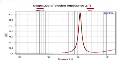
The LPM  $1^{st}$  measurement provides the linear parameters of the driver. The force factor BI(0), the moving mass  $M_{ms}$  and the voice coil resistance  $R_e$  are exported to the  $2^{nd}$  measurement. For manual calculation, the resonance frequency  $f_s$  is required for the assessment of  $X_L$  and  $X_D$  due to inductance nonlinearity and Doppler effect.
