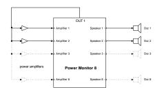
Use a separate amplifier for each DUT if the impedance of the transducers is relatively low and the power amplifier may not provide the current for multiple DUTs connected in parallel.
