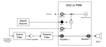
The figure above shows a first application of the manual pilot tone adjustment which is applicable to INTERNAL, BYPASS and EXTERNAL Modes. The user defines the frequency (2 Hz ... 18 kHz) and the fixed amplitude of the pilot tone at XLR connector OUT1 which is superimposed with the internal or external power test signal. Using a fixed pilot tone speeds up the initial phase of the power test. This setup is convenient for power testing of drive units together with the active or passive crossover.
