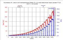
The voice coil temperature (upper curve) is closely related to the real input power (lower curve) supplied to the transducer. Both state variables plotted versus measurement time give important information for defining admissible maximal input power.
