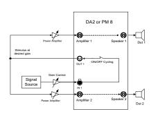
Alternatively, the stimulus from the external signal source may be transferred via IN1 and OUT 1 through the power test hardware to realized ON-OFF cycling in the bypass mode. The PWT software displays the monitored voltage at the loudspeaker terminals and the user adjusts the gain at the signal source or power amplifier to realize the desired target voltage.
