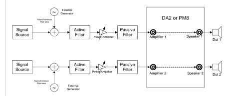
This application shown above uses only external signal sources for power testing. If the stimulus does not provide sufficient spectral density at the frequency  $f_p$  specified in the PP MANUAL PILOT TONE then it is recommended to add a separate pilot tone at the same frequency  $f_p$  which is asynchronous to the analysis performed in the hardware.
