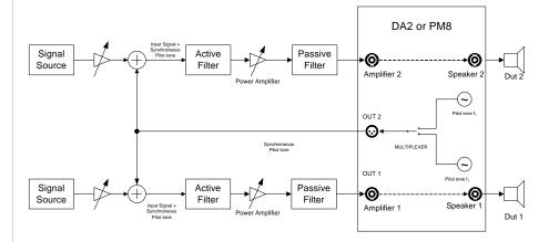
The application in the figure above performs an external mixing of the pilot tone provided at OUT2 of the measurement system with the external power test stimulus before feeding this signal via power amplifier and electrical monitoring to
