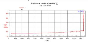
The electrical resistance  $R_e$  of the voice coil increases with the instantaneous voice coil temperature. A sudden increase indicates a loose connection or a broken coil. A sudden decrease is caused by a shortcut of the windings in the gap.
