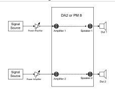
The Bypass mode allows using separate signal sources for each device under test. The voltage at the terminals is controlled manually by changing the gain at the power amplifier until the monitored voltage at speaker terminals fit the target value.
