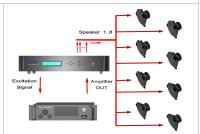
The stimulus (noise, sweep, test tones) is generated internally and supplied at the output XLR connector OUT1. The internal mode controls the amplitude of the stimulus automatically, performs and ON/OFF cycling and a stepping functionality.
