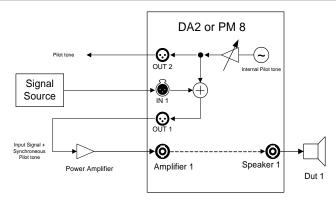
If the checkbox AUTOMATIC PILOT TONE is activated the pilot tone is set to the lowest frequency (2,4,8 Hz) which passes the amplifier's high-pass at sufficient
