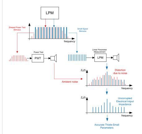
However, a small signal measurement may be corrupted by noise generated by other DUTs tested at full power in a relatively small power test room or climate chamber. The figure above illustrates a technique how to cope with the "microphone effect" by using a power test stimulus in PWT which is incoherent with the small signal stimulus used in the LPM. Those stimuli are two sparse multi-
