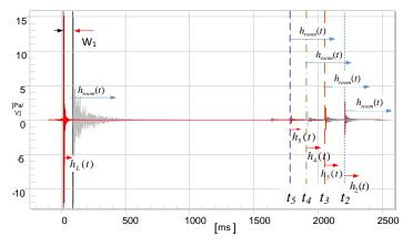
Applying to the microphone signal a filter, which compensates for the room influence reduces the ringing of the impulse response strongly.
