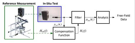
After this initial calibration of the setup, multiple measurement with different stimuli can be performed. The room reflection are compensated in time domain by applying this compensation filter directly to microphone signal. Thereby, this technique can be used for any stimulus and analysis, acquiring accurate measurements of nonlinear distortion and transient responses.
