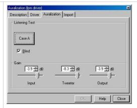
These tests may be performed as blind or even double blind tests to avoid any bias and to check the reproducibility of the results. During the blind test the user has no access to the attenuator for the linear signal and the distortion but may adjust the input, output and tweeter amplitude. The designation Case 1 and Case 2 will be renamed by chance to Case A and Case B in order to hide the setup to the subject. The amplitudes of all
