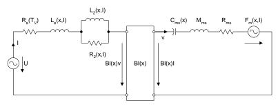
The lumped-parameter model shown above is used to describe the large signal behavior of electro-dynamical drivers at high amplitudes. In contrast to the well known linear model the elements
