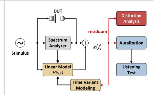
The *Live Audio Analyzer* is a tool dedicated to long-term measurement of active and passive audio systems. It can be used with music, speech or dedicated test signals while monitoring up to five sensor signals simultaneously. For physical and perceptual evaluation of sound quality, the *Live Audio Analyzer* combines modern measurement and listening techniques (auralization).
