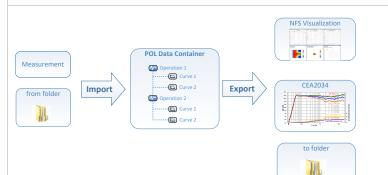
After finishing the measurement all data is stored in a data container in database. This container provides an open export interface for further analysis of the results.
