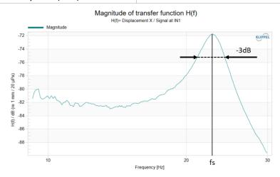
The *TRF* module calculates the transfer function H(f) = X(f)/P(f) which is used to determine the modal resonance frequency  $f_s$  and 3 dB bandwidth  $\Delta f_{3dB}$ . From these values, the geometrical parameters of the beam and its mass the modal E modulus and loss factor  $\eta$  are calculated. The calculation is done by using the CAL-module.
