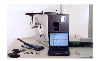
The material parameter measurement module (MPM) measures the Young's E modulus and the loss factor  $\eta$  of the raw material used for loudspeaker design. The vibration beam technique (ASTM E 756-93) is modified to be capable for measuring also soft materials such as thin foils of plastic, rubber and any kind of paper and impregnated fabric. After cutting 1 cm strips the probes are clamped on one side and excited pneumatically by using the suspension part measurement bench.
