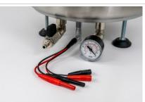
The DUT will be connected with standard laboratory 4 mm connectors, which are fed inside the chamber through vacuum-tight 4-pin LEMO couplers.
