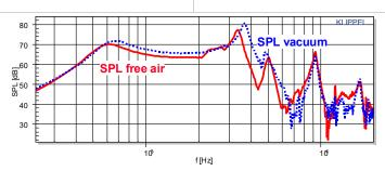
SPL response of a headphone predicted by using cone vibration measured in free air (solid line) and in vacuum (dotted line). Note that the moving mass of the air load shifts the natural frequency of the first bending mode from 3.8 kHz found in vacuum down to 3.4 kHz in air and causes a different vibration pattern as shown below.
