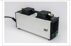
Klippel offers an oil free diaphragm vacuum pump for laboratory use. The oil free diaphragm technique requires no maintenance. Typical evacuation time to reach -0.9 bar in the Klippel 7 liter vessel is about 140 s with the default vacuum pump and less than half the time with the extended capacity vacuum pump.
