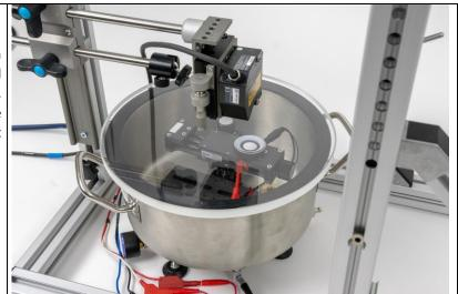
The stand supports the operation of the laser sensor in horizontal (default) and vertical direction, e.g. for vacuum measurements with the additional vacuum measurement chamber. The stand could also be used to position sensors to external test objects.
