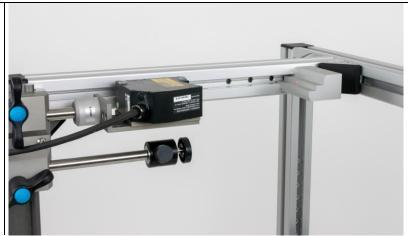
For laser sensors with less than +/- 12 mm measurement range a Translation Stage with a high-resolution micrometer is a required accessory for calibration.
