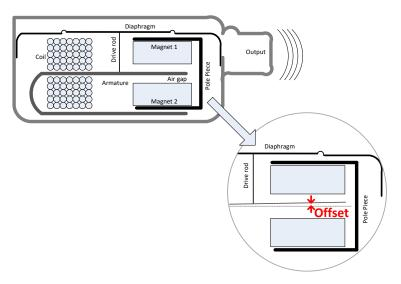
Fig. 1: Schematic view of the armature offset.
