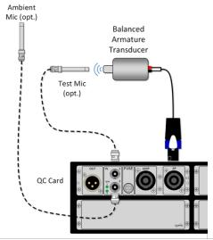
The figure shows the minimal equipment required to run the BAC:
