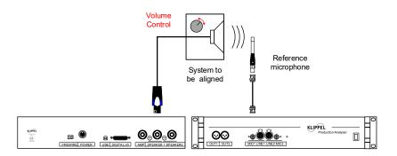
A simple application of the EQA is level adjustment of an active or passive speaker's response at a defined frequency or based on average level in a certain frequency band. Using a calibrated microphone, the desired target SPL is manually adjusted by the operator while the EQA compares the response to the target level and terminates the test when the target is reached within the specified tolerance.
