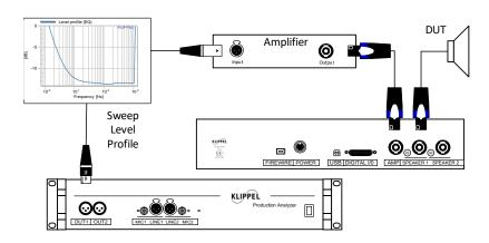
Typical audio amplifiers suffer from a high-pass characteristic at very low frequencies resulting in gain decay. The EQA may be used to determine and compensate this characteristic. By this, consistent excitation of the DUT can be assured within the complete tested frequency range.
