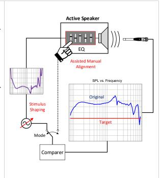
The QC Equalization + Alignment is a versatile tool for adjusting the level or frequency response of transducers, audio systems or electronics.
