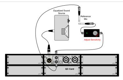
The EQA may be used for manual sensitivity adjustment at a defined frequency or based on average level over a full frequency band. This can be used to adjust preamplifier factory settings of a microphone or an audio device that provides integrated microphones (e.g. smart speaker).
