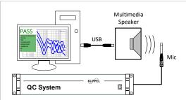
The stimulus is played back with a USB audio device with unknown delay. The synchronization is performed dynamically through the acoustical measurement channel. Subsequent measurements use the detected delay to trigger the analysis in the quasi-synchronous playback process.
