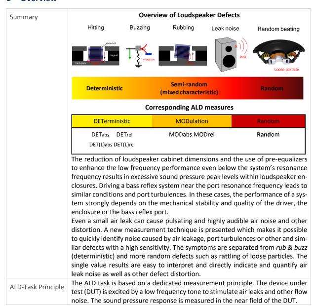
The output parameters of the ALD task are calculated by exploiting the unique signal characteristics of amplitude modulated air noise and deterministic leak distortion, which also provide separation from other defects and uncorrelated signals.
