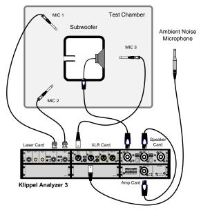
The stimulus signal is played back only once by the source ALD task that simultaneously captures all other microphone signals. The receiver tasks only process the microphone signals recorded by the source tasks in order to generate the test results and verdicts for all microphones.
