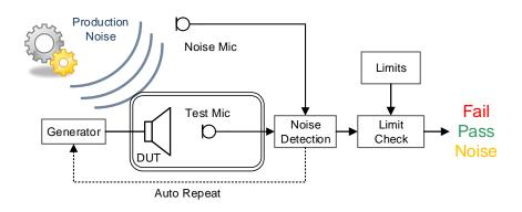
**Note**: The integrated leak detection in the SPL task may be combined with *the Production Noise Immunity* option. Without this option, ambient noise corruption is still reliably detected. Please see specification *S21 - QC Production Noise Immunity*.
