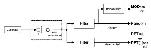
SPL-Task Integration The same analysis methods can be applied to a defined frequency band of the standard SPL sweep for parallel analysis of leak symptoms and standard acoustical properties. A user defined center frequency and bandwidth define a part of the sweep which is analyzed for leak symptoms. The results are identical to the ALD-task with the exception of Random symptoms. Such are detected in the SPL-Task using the standard Rub&Buzz measure.
