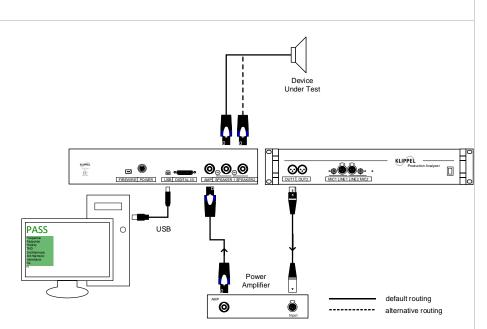
The figure above shows the minimal equipment required to run the MSC with KLIPPEL Production Analyzer:
