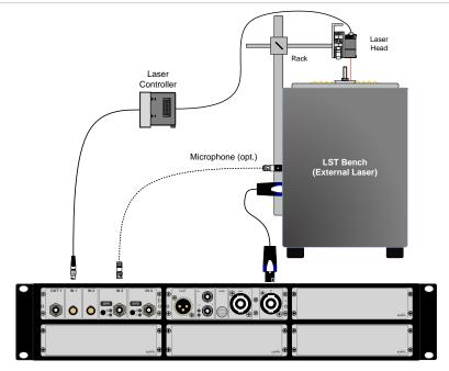
The schematic above shows a simplified alternative hardware setup with *Klippel Analyzer 3* (*KA3 LQ*) hardware, *LST Bench* with external laser mounting and *LK-H52* laser set.
