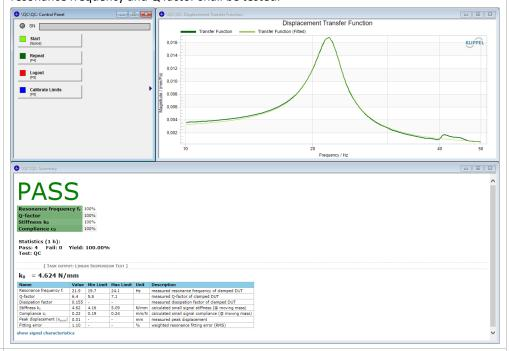
LST Pro (Item # 4000The LST Pro extends the Lite version with additional signal processing and two more results: mass deviation and stiffness deviation (relative to Golden DUT). The LST Pro is dedicated for advanced testing of passive radiators identifying the root cause of
