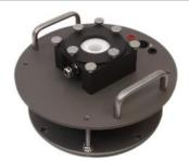
The MSPM bench add-on is dedicated to testing small diaphragms with higher resonance frequencies. It is an extension for the LST bench with external laser mounting. It provides a dedicated mounting platform for custom made DUT carries, a microphone mount and a built-in speaker.
