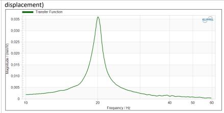
The resonance frequency is read at maximal amplitude, Q factor is defined by -3 dB drop.
