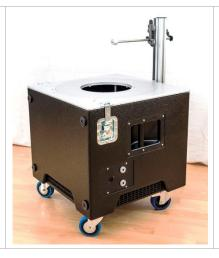
The LST Bench is capable of handling test objects up to a diameter of 222 mm which corresponds to the largest ring of the optional clamping ring set.
