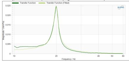
For large size test objects resonance may be hardly detectable in displacement. Therefore, sound pressure measurement might be mandatory.
