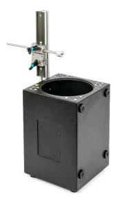
This bench is an extended version of the LST Bench providing an external laser boom. The laser is mounted externally for faster adjustment in case of frequently changing DUTs.
