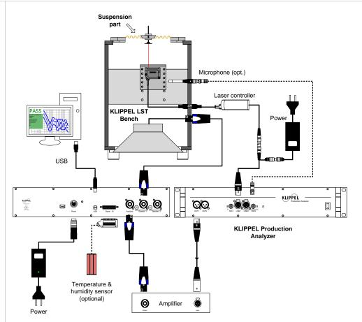
The figure above shows the equipment required to run the LST
