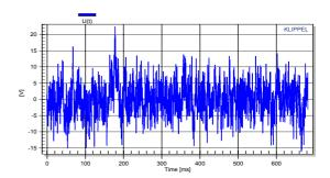
Fig 5: Measured voltage u(t) versus time t of the stimulus at the loudspeaker terminals by using a multi-tone stimulus
