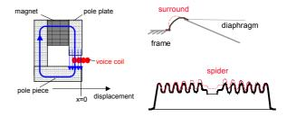
Fig 1: Loudspeaker nonlinearities caused by manufacturing: Offset in the voice coil rest position (left) and variation of the suspension geometry (right)
