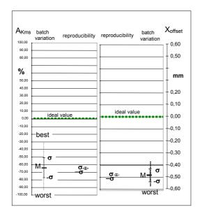
Fig 19: Mean value M, standard deviation  $\sigma$  and the the values of the Stiffness asymmetry  $A_K$  and voice coil offset  $x_{offset}$  measured by the new MSC method on the complete batch. The reproducibility is tested by repeating 30 times the measurement on one single device.
