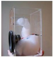
Fig 9: Damping material in the port of a vented-box system.
