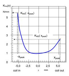
Fig 15: Reading the suspension asymmetry  $A_K$  from the nonlinear  $K_{ms}(x)$  curve measured by conventional LSI technique.
