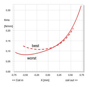
Fig 17: Stiffness characteristic  $K_{ms}(x)$  versus displacement x of the best and worst headphone unit measured by the conventional LSI method.
