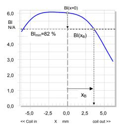
Fig 11: Reading the maximal peak displacement  $x_B$  limited by force factor only (Bl(x)-curve is measured by conventional LSI technique).
