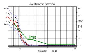
Fig 16: Mean value, standard variation and best and worst curve of the total harmonic distortion measured at 30 headphone drive units.
