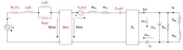
Fig 3: Electro-mechanical equivalent circuit of a vented-box system
