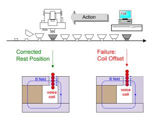
Fig 20: Measurement of the voice coil offset at the end-of-line testing and adjustment of the manufacturing process.
