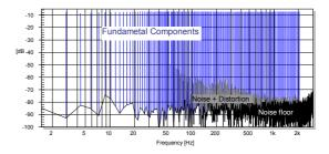
Fig 6: Spectrum U(f) of the measured voltage at the loudspeaker terminals by using a multi-tone stimulus
