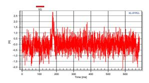
Fig 7: Electrical current *i(t)* measured at the loudspeaker terminals by using a multi-tone stimulus.
