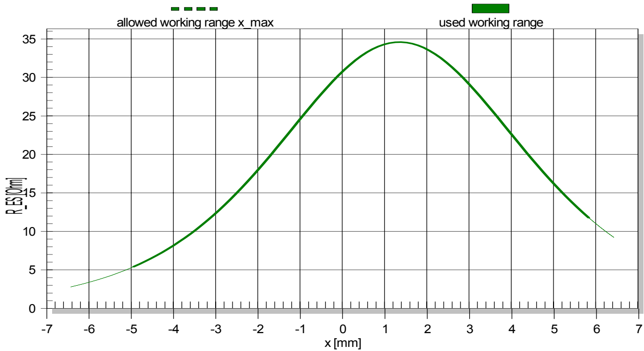
Fig. 17: Resistance R_{ES}(x) representing the mechanical losses in the electrical equivalent circuit depending on voice coil displacement due to transformation with nonlinear force factor b(x) .
