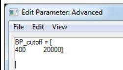
The delivered example uses a band-pass with cut-off frequencies 400 Hz and 20 kHz.
