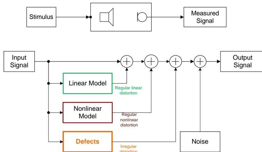
The regular linear distortion can be predicted by lumped or distributed parameters of the linear transducer model. The linear distortion generation is optimized during the design process. Another linear distortion is the influence of the listening conditions (room acoustics).
