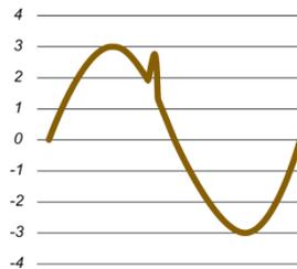
4. Let's calculate the difference signal. We get the peak, which is very good since this is the thing we're interested in. Also we get a sinusoidal component, which is only due to amplitude compression. Since this is a natural self-protection of the loudspeaker we're not so interested in getting that component in the auralization output.
