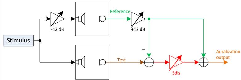
This way parasitic vibration is isolated. The regular nonlinear distortion component is also contained in the difference signal but is neglected in this case (see *Filtering*).
