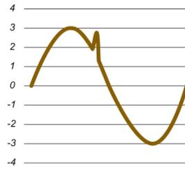
d. For  $S_{dis}>0$  dB, the peak is enhanced, but the sine component is reduced even further ...
