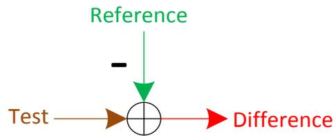
The input signals have to be aligned in time and level before the subtraction. The time alignment is performed automatically by the DIF-AUR, thus providing synchronous signals.
