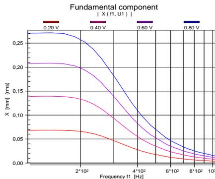
The fundamental of the excursion shows the typical roll off of 12 dB / octave above  $f_s$ . Compression effects are hardly detectable. See also the Compression window in DIS.
