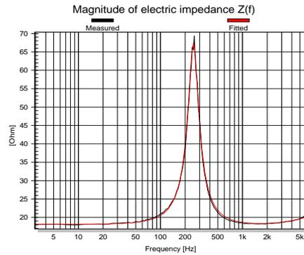
This driver has a high impedance peak, indicating sufficient back induced voltage for parameter identification both in LPM and in LSI.
