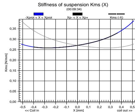
The stiffness (inverse of compliance) has a significant asymmetry. This causes not only a 2<sup>nd</sup> order harmonic distortion in sound pressure ( $f \leq f_s$ ) but generates also a dc component  $X_{dc}$  in displacement directed to negative displacement (where the stiffness is lower).
