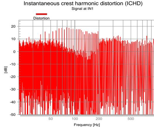
Exciting the driver with a sine sweep of 0.9V suddenly impulsive distortion are generated between 50 Hz and 200 Hz which have a crest factor which is much higher than the crest factor (about 12 dB) found at other frequencies.
