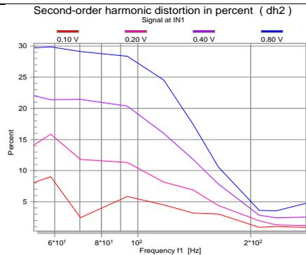
The asymmetry in the stiffness curve  $K_{ms}(x)$  generates cause most of second order distortion below the resonance frequency.
