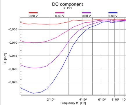
The measured DC part is generated by the asymmetry in the stiffness curve  $K_{ms}(x)$ . This DC part shifts the working point dynamically to negative displacement where the stiffness is lower.
