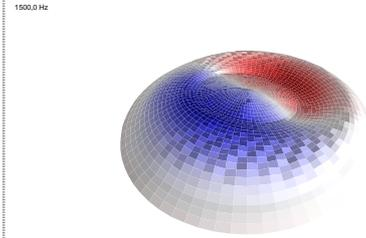
3D view of the geometry and superimposed vibration (blue and red indicates opposite directions) of a rocking mode
