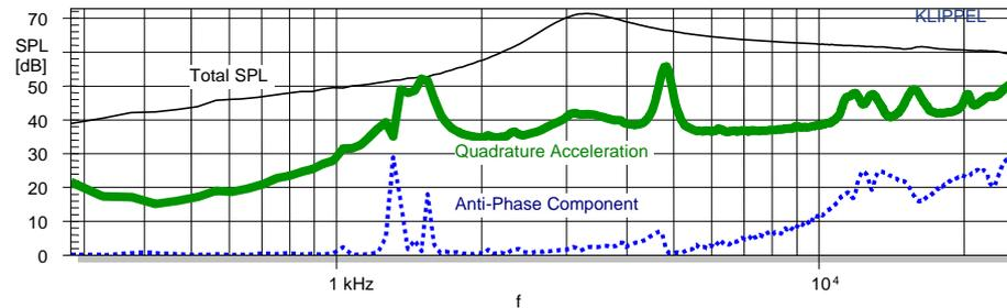
The geometry and vibration data measured by laser scanning are valuable parameters of the microspeakers in addition to linear and nonlinear parameters. They are the basis for predicting the sound pressure output at any point in the far field as shown as black solid line (**Total SPL**) in the figure above.
