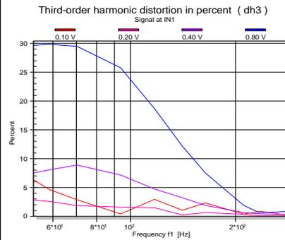
3<sup>rd</sup> –order harmonic distortion are generated by the symmetrical decay of  $Bl(x)$  and symmetrical increase of  $K_{ms}(x)$ . Suddenly at 0.8V the 3rd order distortion comes up due a hard limiting effect of the  $K_{ms}(x)$ .
