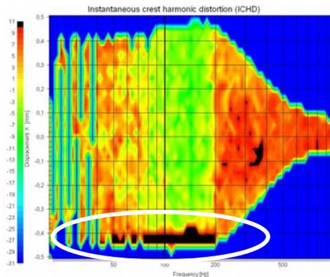
The instantaneous crest factor of the higher-order distortion represented as colour in left figure can be plotted versus frequency (x-axis) and voice coil displacement (y-axis). If the colour becomes black the crest factor is larger than 12 dB indicating impulses with high peaks.
