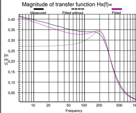
The Creep effect has to be considered in the measurement of the linear parameters to reduce the fitting error in the displacement transfer function  $H_x(f)$ .
