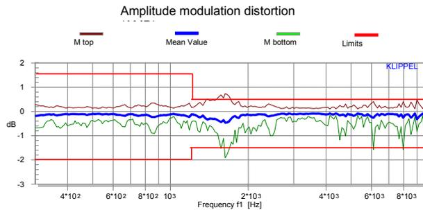
The top and bottom modulation  $M_{top}$  and  $M_{bottom}$  describe the minimal and maximal variation of the envelope. The mean modulation shows the variation of the amplitude response of the high frequency tone with and without bass tone.
