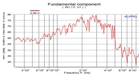
After performing the reference measurement with the voice tone  $f_1$ , the window **Fundamental** shows the amplitude response of the high frequency voice tone  $f_1$  versus frequency.
