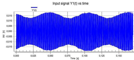
This variation of the envelope shows a pure amplitude modulation of the voice tone  $f_1$  according to frequency  $f_2 = 20$  Hz.
