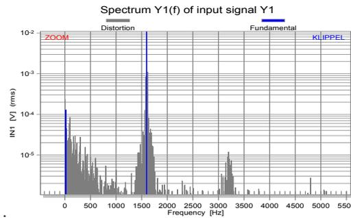
The bass tone at  $f_2=20$  Hz causes harmonic distortion at lower frequencies and intermodulation centered around the voice tone at  $f_1 = 1600$  Hz. The distortion above 3 kHz are harmonics of the voice tone  $f_1$ ,
