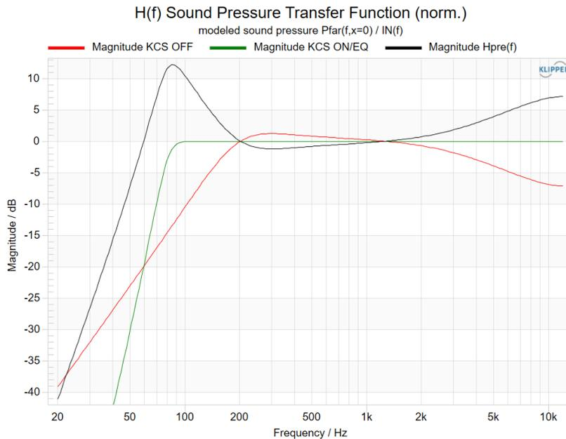
This window shows the predicted small signal sound pressure transfer function of the target system before and after applying the pre filter  $H_{pre}(f)$  which contains a linear alignment filter and a linear inductance compensation filter. The transfer functions are normalized so that a gain of 0 dB at high frequencies is reached for a virtual loudspeaker system without inductance. See [1.6](#) and [2.3](#) for detailed information.
