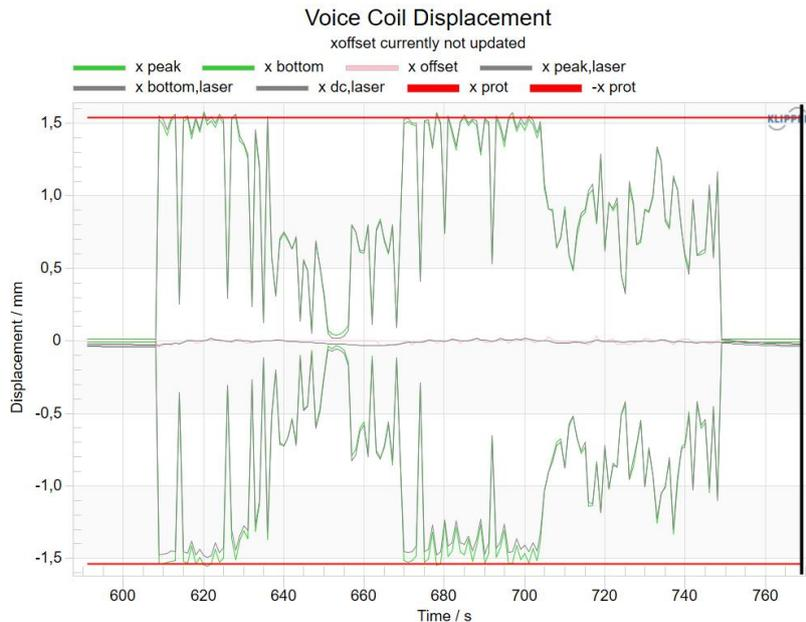
The window *Displacement* shows the absolute voice coil displacement over time. This information is e.g. important for evaluating the functionality of the mechanical protection system. The green curves represent the positive and negative peak displacement.
