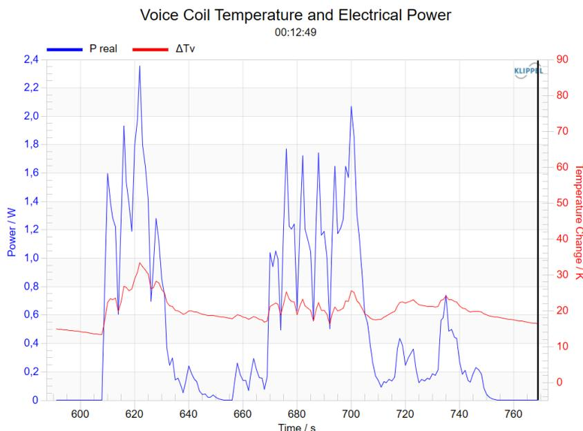
This window shows the increase of the voice coil temperature  $\Delta T_V$  and the electric input power  $P(t)$  versus time. This information is very helpful to verify that the transducer's power handling and the amplifier dimensioning is sufficient.
