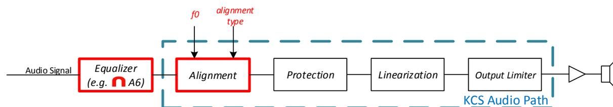
The automatic alignment feature of KCS allows to tune the low frequency response of the system to a desired transfer function with defined cut-off frequency  $f_0$  and filter type (such as *Butterworth* or *Chebyshev*). Due to the adaptive compensation of time-varying speaker parameters, this transfer function will be maintained over the whole lifetime of the transducer. The Alignment is used to
