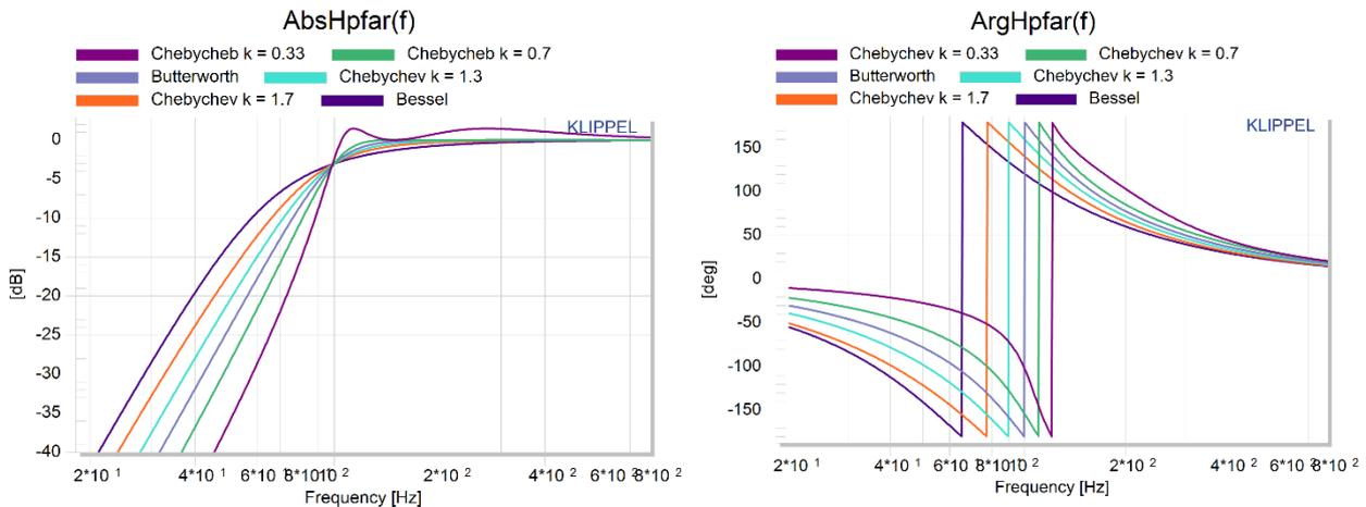
Magnitude and Phase of the target responses for various 4<sup>th</sup> order alignments with a cut-off frequency of 100Hz.
