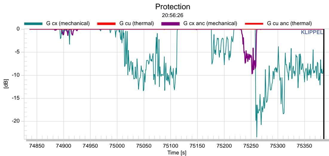
In the *Protection* Chart, the audio and the ANC signal attenuation gains are shown separately. If the assigned ANC budget is exhausted, the ANC protection is activated.
