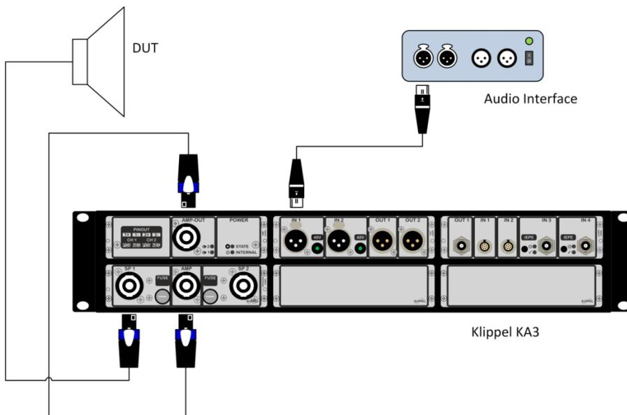
Hardware connection on KA3 with AMP Card
