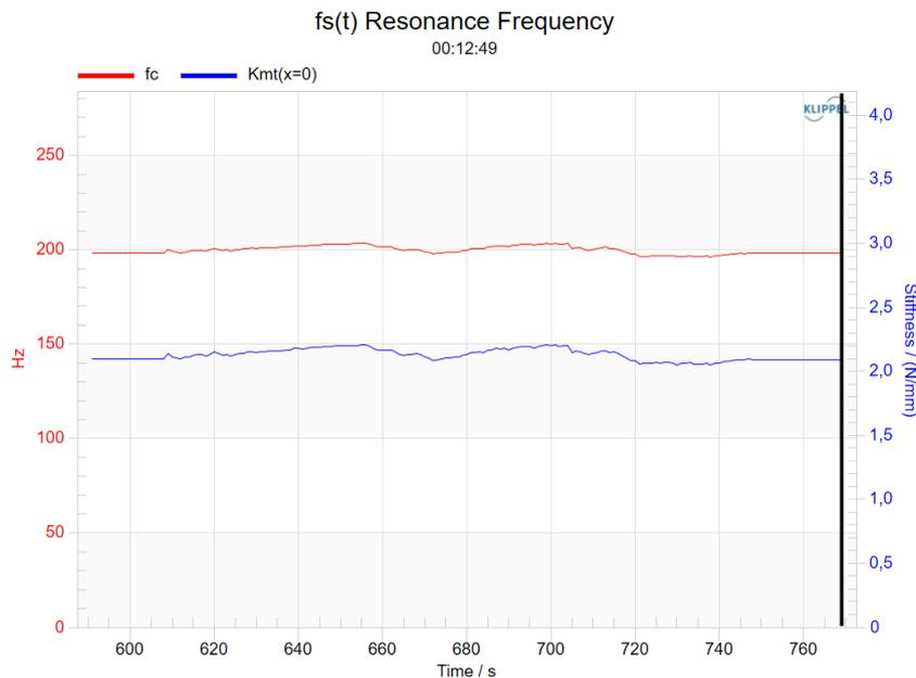
This result window shows the speaker's resonance frequency  $f_s(t, x=0)$  or  $f_c(t, x=0)$ , the stiffness of the mechanical suspension  $K_{ms}(t, x=0)$  or  $K_{mt}(t, x=0)$  at the rest position  $x = 0$ .
