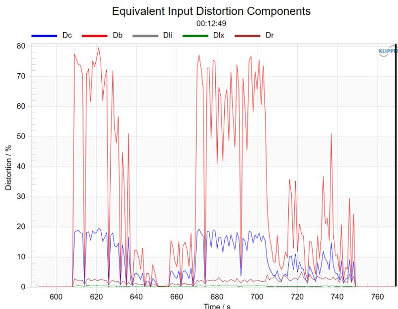
The relative distortion components describe the ratio of the peak values of the *equivalent input distortion* generated by the selected nonlinearities and the peak value of the total signal.
