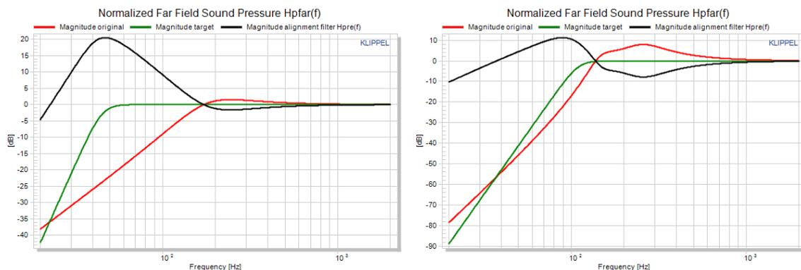
Alignment Transfer Functions. Applying alignment sealed box (left) and a passive radiator box system (right). The green curves represent the target response.
