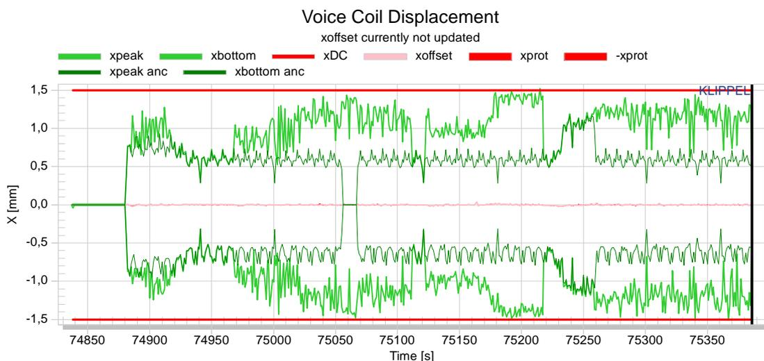
Right-click inside the voice coil displacement chart and select “Show all curves” to see the separate displacement caused by the ANC input signal only. The ANC displacement budget is fixed to 70% of the available displacement working range (xprot).
