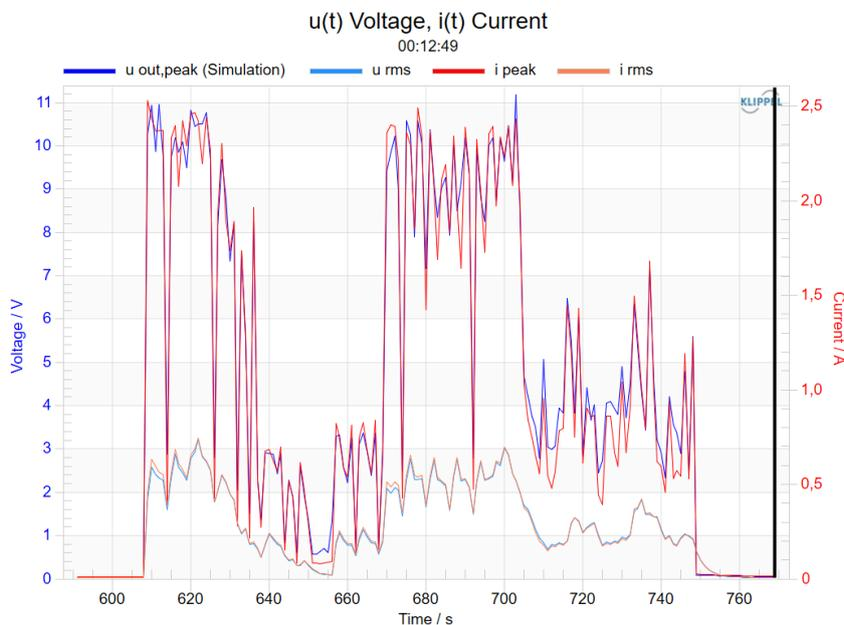
The voltage and current signals are essential for dimensioning a proper amplifier for the particular application. For amplifier evaluation, it is very useful to evaluate the peak values of voltage and current with different signals (e.g. different music signals, speech) and different alignments for verifying that the amplifier is sufficiently dimensioned, esp. in regards to peak voltage capability. For
