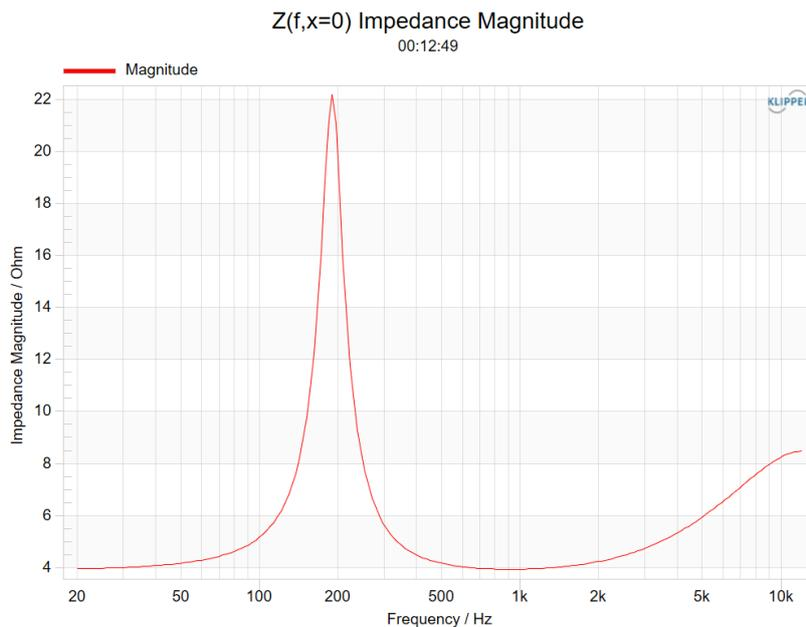
The impedance magnitude is calculated based on the identified linear speaker parameters.
