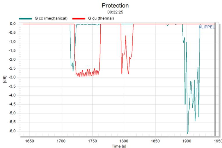
The activation of the mechanical and thermal protection systems can be observed at any time. The attenuation value  $G_{cx}$  (*mechanical*) indicates an approximate value at which degree low frequencies are attenuated. The attenuation value  $G_{cu}$  (*thermal*) indicates the attenuation value of how much the whole audio signal is attenuated. See more information in the tutorial [1.7.1](#).
