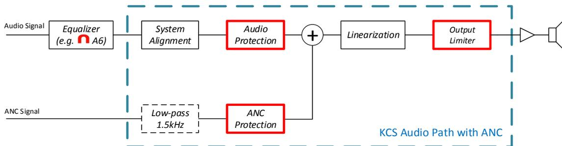
**Note:** The fixed low-pass filter in the ANC Signal is only available upon special request and is preferably applied externally prior to any KCS processing. The currently implemented 4<sup>th</sup> order Butterworth filter at 1.5kHz adds 0.3 ms group delay to the ANC processing.
