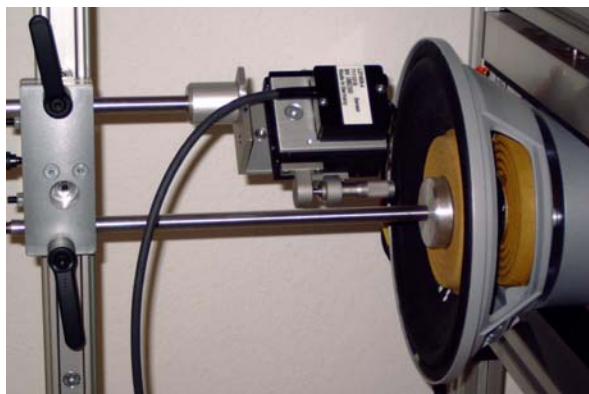
Figure 4 Generating an additional DC offset by the lower rod connected by an addition spider to the diaphragm.
