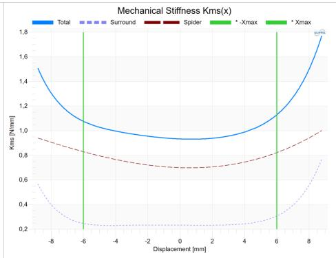
The nonlinear stiffness  $K_{ms}(x)$  versus displacement x can be measured over a wide amplitude range by using the initial identification (KCS-ID) and KLIPPEL LSI module.
