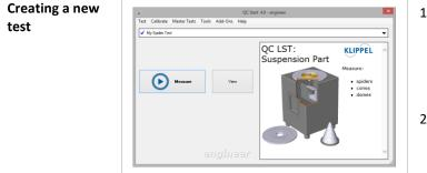
Create a new test by opening QC Start in Engineer mode and selecting *Test – New...*
