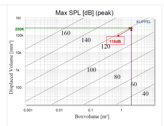
The figures above show an example of testing a subwoofer with a diameter of 140 mm and 18 mm peak displacement. The resulting peak SPL is about 118 dB. An optimal microphone for this application is the MIC255 (AN 2400-009) 1/2" type.
