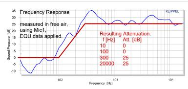
See the QC user manual in the section Optimizing Performance / SPL Tests / How to cope with ambient noise? / How to measure Box attenuation? on how to calculate the specific ambient noise attenuation of the test box and how to set up the test setup considering this attenuation.
