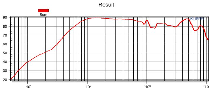
Within the frequency limit  $f_{NF\max}$  this result is not corrupted by the acoustical environment and can be converted to an equivalent far field response.
