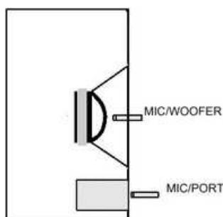
The measurement microphone should be placed normal and as close as possible to the center of the dust cap to ensure a quasi-anechoic measurement caused by the high level differences between direct sound and room reflections. By keeping the micro-phone distance less than 11% of the effective radius  $a$  of the cone, the measurement error will be less than 1dB.
