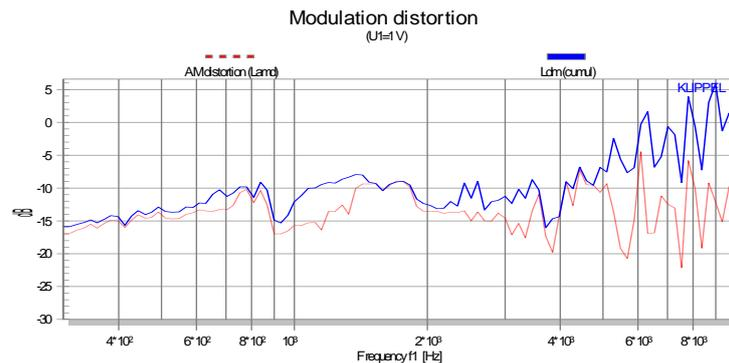
The solid curve shows the distortion  $L_{dm}$  caused by amplitude and frequency modulation. The dashed curve shows the distortion  $L_{AMD}$  caused by amplitude modulation only. Clearly, the AM modulation is dominant at low frequencies while the frequency modulation mainly caused by the Doppler effect is about 15 dB higher at high frequencies.
