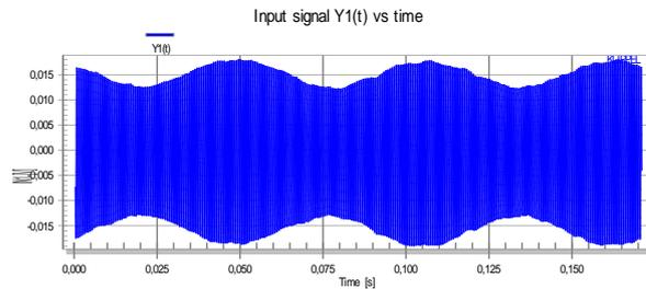
This variation of the envelope shows a pure amplitude modulation of the voice tone  $f_1$  according to frequency  $f_2 = 6$  Hz.
