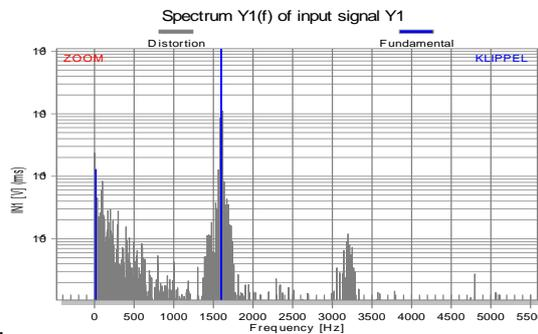
The bass tone at  $f_2=6$  Hz causes harmonic distortion at lower frequencies and intermodulation centered around the voice tone at  $f_1 = 1600$  Hz. The distortion above 3 kHz are harmonics of the voice tone  $f_1$ ,
