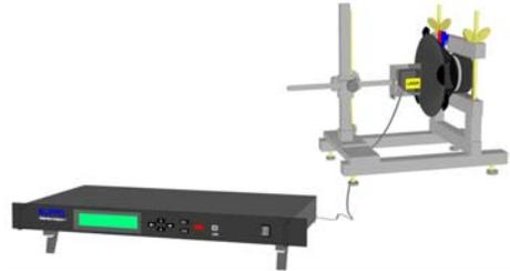
The Distortion Analyzer equipped with a Laser displacement sensor gives the full functionality of a Laser Displacement Meter. It provides the analog displacement signal at the output connector at full bandwidth and displays the results of signal statistics selected at the key pad.
