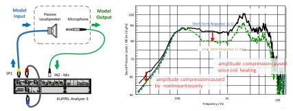
Applications include the investigation of heating effects, the drift of transfer function and durability tests.
