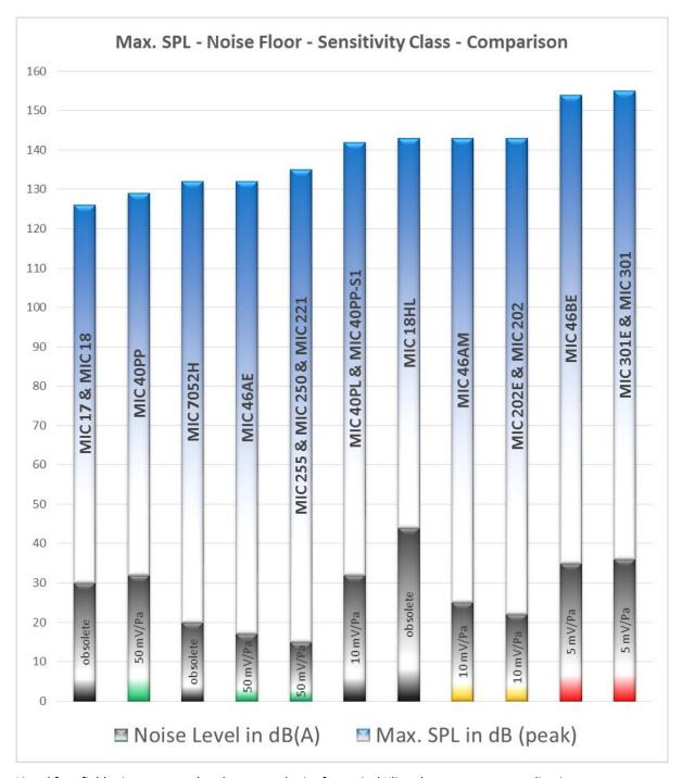
Listed free field mics are tested and suggested mics for typical Klippel measurement applications.
