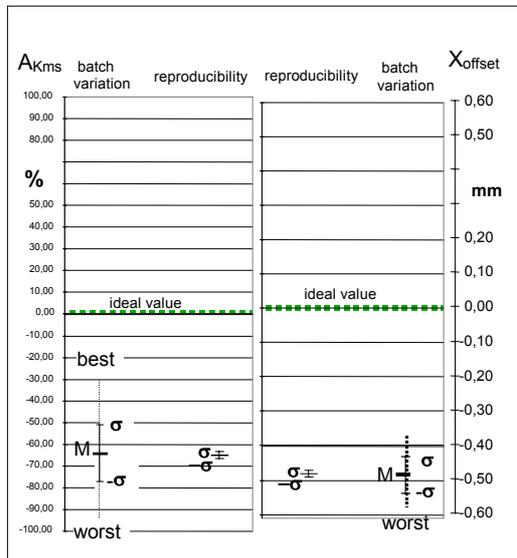
Fig 19: Mean value  $M$ , standard deviation  $\sigma$  and the values of the Stiffness asymmetry  $A_K$  and voice coil offset  $x_{offset}$  measured by the new MSC method on the complete batch. The reproducibility is tested by repeating 30 times the measurement on one single device.
