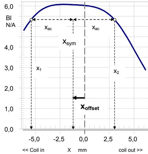
Fig 12: Reading the voice coil offset  $x_{offset}$  from the symmetry point in the nonlinear  $Bl(x)$ -curve measured by LSI.
