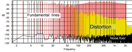
Fig 8: Spectrum  $I(f)$  of the measured current at the loudspeaker terminals by using a multi-tone stimulus
