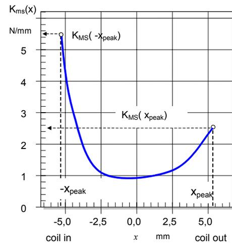
Fig 15: Reading the suspension asymmetry  $A_K$  from the nonlinear  $K_{ms}(x)$  curve measured by conventional LSI technique.
