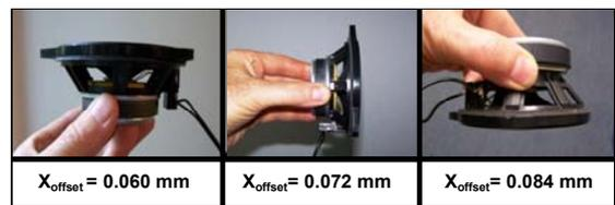
Fig 13: Measurement of the influence of gravity on the voice coil offset  $x_{offset}$ .
