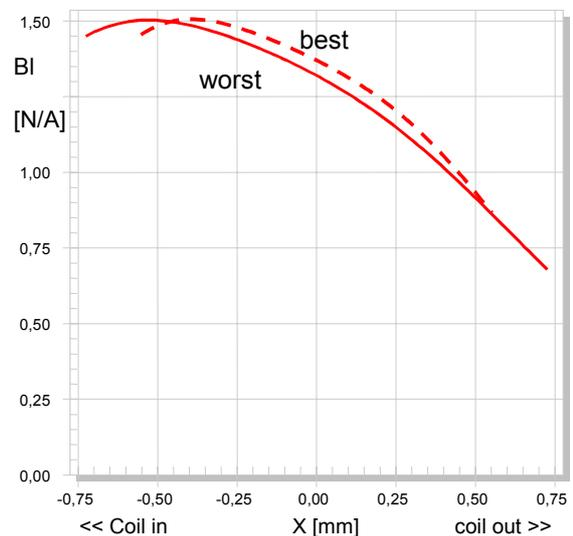
Fig 18: Force factor characteristic  $Bl(x)$  versus displacement  $x$  of the best and worst headphone unit measured by the conventional LSI method.
