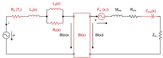
Fig 2: Electro-mechanical equivalent circuit of a drive unit
