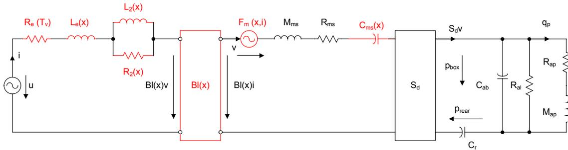
Fig 3: Electro-mechanical equivalent circuit of a vented-box system
