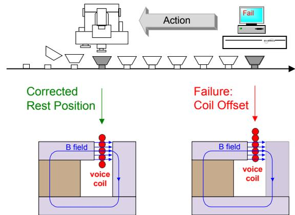
Fig 20: Measurement of the voice coil offset at the end-of-line testing and adjustment of the manufacturing process.
