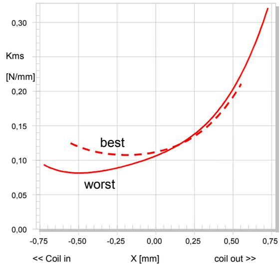
Fig 17: Stiffness characteristic  $K_{ms}(x)$  versus displacement  $x$  of the best and worst headphone unit measured by the conventional LSI method.
