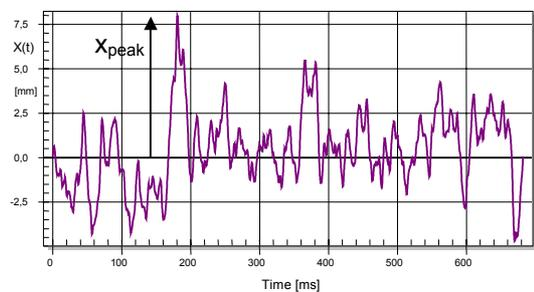
Fig 10: Voice coil displacement  $x(t)$  versus  $t$  predicted by the large signal model.
