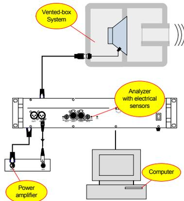
Fig 4: Setup for the measurement of the large signal parameters of a vented-box system by using electrical sensors only.
