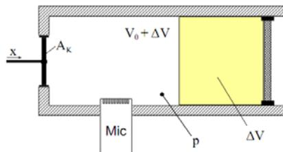
Using two measurements in different volumes it is not necessary to determine the absolute volume  $V_0$  of the air in the enclosure where the driver is mounted. The absolute volume is replaced by the variation  $\Delta V$  of the air volume.
