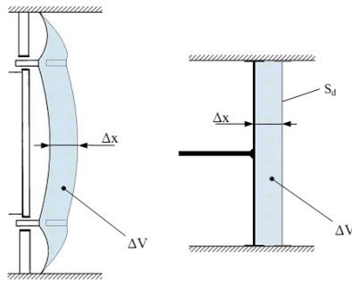
At sufficiently low frequencies every loudspeaker can ideally be represented as an infinitely rigid piston, which displaces the same air volume  $\Delta V$  at a constant voice coil displacement  $\Delta x$ . The area of this piston is always smaller than the real cone area and it is characterized as the effective radiation area  $S_d$  with the effective radius  $r_d$ .
