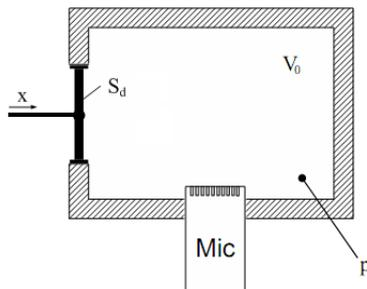
A pistonphone is usually used as an apparatus for microphone calibration. It simply consists of a closed volume  $V_0$  producing an acoustical compliance  $N_a$  and a rigid piston with the surface  $S_d$ . Sinusoidally excited with a constant peak displacement  $x$  the piston generates a constant peak sound pressure  $p$  inside the volume using
