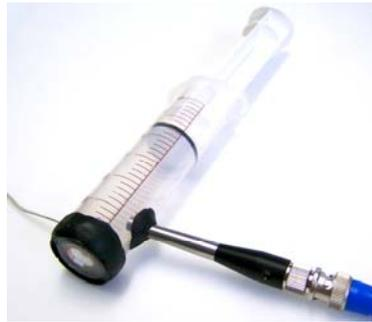
Because of the intricate construction of the driver we recommend to perform two measurements in different volumes if you do not know the volume of the driver. A quite simple possibility for a microspeaker is using a syringe, which allows an easy metering of the volume difference. You may cut off the orifice to place the driver and drill two holes for the microphone and the cables. We recommend using a second volume which is about 1.5 to 3 times as big as the first one.
