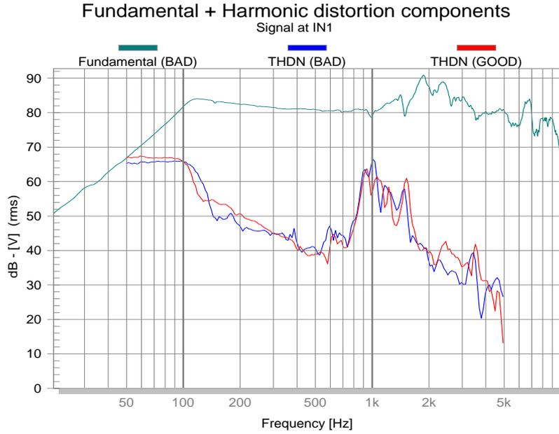
For comparison the THD curves of a good and a bad driver are presented. It is obvious that the THD is not a suited measure to describe and detect R&B phenomena. The regular distortion, caused by motor and suspension nonlinearities, mask the much smaller rub & buzz distortion.
