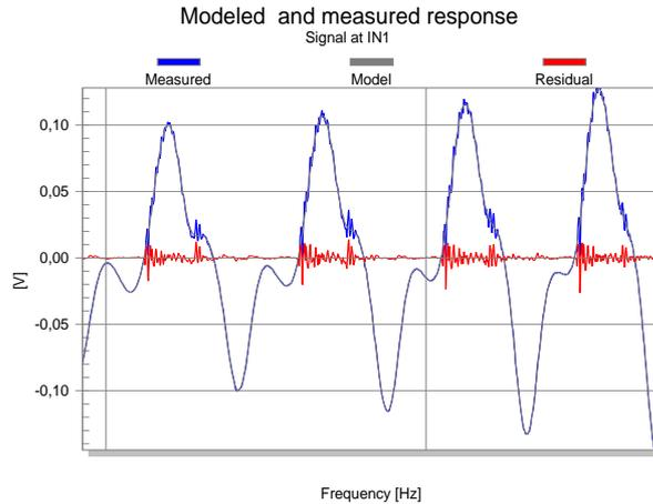
The red curve in the result window Modeled Rspose shows the instantaneous distortion  $e(t)$  in the time domain signal. Impulsive distortion are only generated for a half wave of the measured, non-processed time signal  $y(t)$  represented as blue curve. Clearly the defect only occurs for positive displacement of the voice coil.
