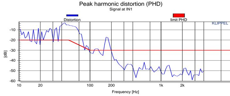
The second operation *TRF Crest Harmonics* ( $x, f$ ) shows the Peak value PHD of the harmonic distortion. The PHD is higher than the allowed limit value for frequencies at 20-150 Hz where the Crest factor is above the limit. The impulsive distortion has a high impact on sound quality.
