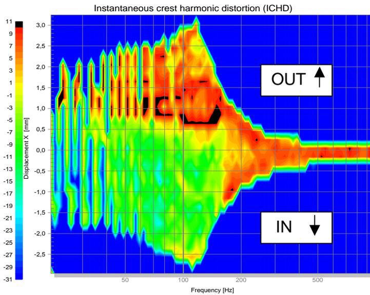
The result window Instantaneous Distortion 3D shows the crest factor ICHD (as color) versus voice coil displacement (y axis) and frequency (x axis). This reveals valuable information about the location of the R&B defect. Black spots at frequencies 20-150 Hz and for positive voice coil displacement indicate a voice coil rubbing.
