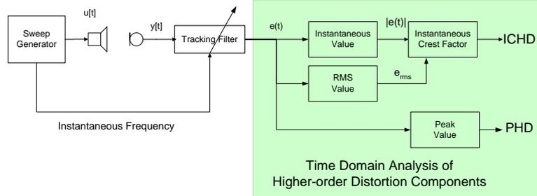
The rub & buzz detection algorithm is based on a time domain analysis to overcome the disadvantages of the THD measure and to show impulsive distortion at high temporal resolution.
