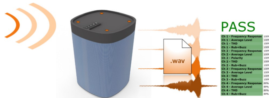
Figure 4: Wave file-based testing a smart speaker's four microphone responses using KLIPPEL QC.
