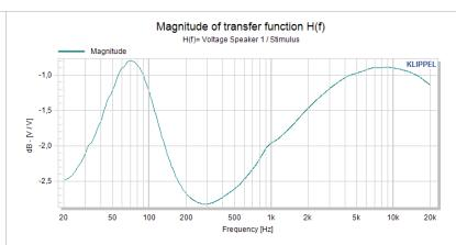
The KLIPPEL Analyzer hardware provides a four-wire sensing technique to measure the precise voltage at the DUT terminals. The deviation between target voltage and real voltage at the terminals is not critical if a linear transfer function is measured in the small signal domain and the output signal (pressure) is divided by the input signal (voltage at the terminals). However, a deviation of 0.5 dB may cause already a significant error in the measurement of nonlinear distortion.
