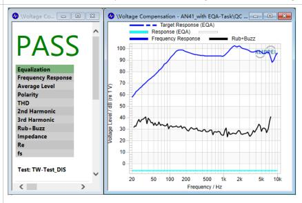
The equalized voltage response can be achieved with the EQA task and is shown in dB in the result window *Frequency Response* (the lower bright blue curve). It can be then applied to the loudspeaker in the SPL task and the corresponding frequency response is measured by the microphone and shown in the same result window (the upper blue curve). Other results such as THD, harmonics and average level can also be measured by activating them as results in the SPL task.
