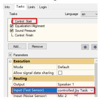
3) Select the EQA task and enter your *Target Response* and the *Tolerance Profile* in section **Configuration**. Please refer to the manual of the EQA task for further information about these parameters.
