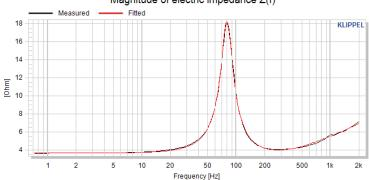
The electrical input impedance Z<sub>D</sub> of the DUT varies significantly versus frequency due to the effect of the mechanical resonance and the electrical inductance of the voice coil. Thus, the current flow through the speaker cable varies a lot over frequency (low current at resonance and at higher frequencies).
