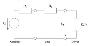
Equivalent circuit explaining voltage variation at the terminals
