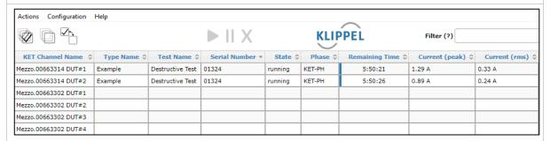
The **Dashboard** is a control panel for managing multiple KET tests. It uses a table-like layout to give an overview about all tests (running, stopped or paused) and is the hub tool for creating new tests. Every row represents one test object operated at one KET channel, which can be labelled by the user.
