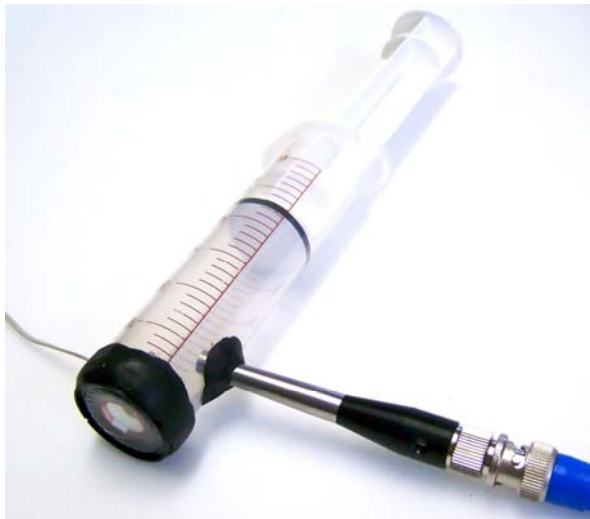
Fig. 6: Performing a differential measurement of the effective radiation area of a headphone by using a syringe.
